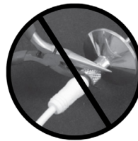
Never use pliers or other tools to tighten the connector
