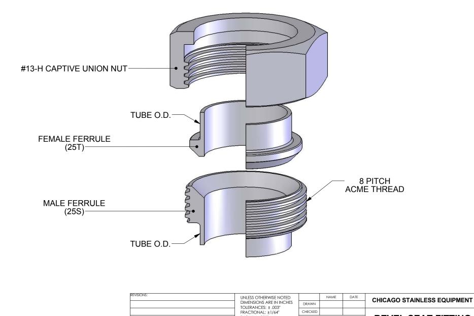
**BEVEL SEAT FITTING** RADIAL: ±.001" COMMENTS: ANGULAR: ±1/4° **ASSEMBLY** REMOVE ALL BURRS **MEASURE TUBE** MATERIAL O.D. TO OBTAIN PROPRIETARY AND CONFIDENTIAL **FITTING SIZE** THE INFORMATION CONTAINED IN THIS DRAWING IS THE SOLE PROPERTY OF **BEVEL SEAT** CHICAGO STAINLESS EQUIPMENT. ANY REPRODUCTION IN PART OR AS A WHOLE WITHOUT THE WRITTEN PERMISSION OF CHICAGO STAINLESS EQUIPMENT IS DO NOT SCALE DRAWING PROHIBITED. SCALE:1:1 WEIGHT: SHEET 1 OF 1
